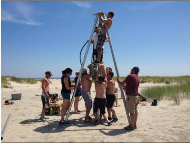
Students operate the Vibracore soil sampler rig used in soil analysis
